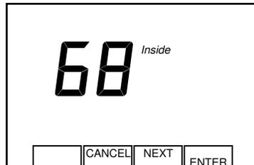
Press the Enter key to save the calibration and return to normal thermostat operation.
