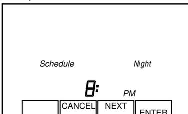
Press the Next key to set the minute for starting Nighttime operation.
