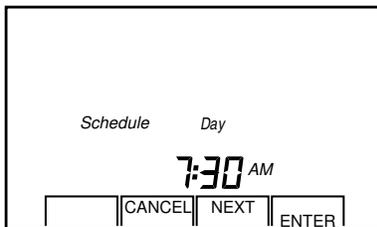
Press the Next key to set the hour for ending Daytime operation and starting Nighttime operation.
