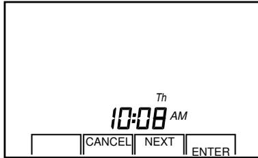
Press the Enter key when complete. The display returns to the normal time and temperature display.
