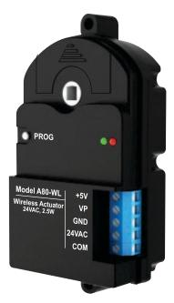
The A80-WL provides a low cost actuator that can be used with dampers up to 12-inch diameter and 1-inch of static pressure. The actuator uses 24VAC power and is controlled remotely using the handheld Remote Control or the Wireless Thermostat.
