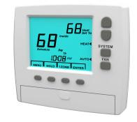
The wireless, battery operated thermostat controls the damper/actuator based on the setpoint temperature, space temperature and the supply air temperature (heating or cooling). The damper is opened or closed proportional to the differential between space and setpoint temperatures and is continually adjusted to keep the space temperature at the setpoint.
